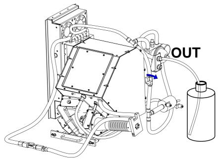
Image 2-3 Drain complete circuit
